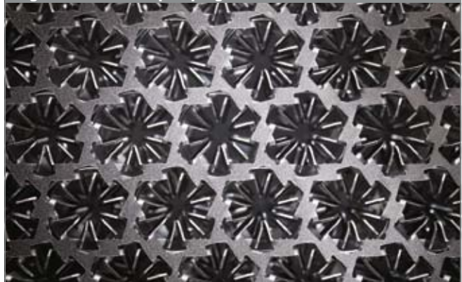
Figure 9 - StarCell pumping element
